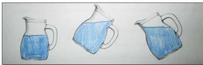
a) Appropriate inclination and the horizontality of the liquid surface
